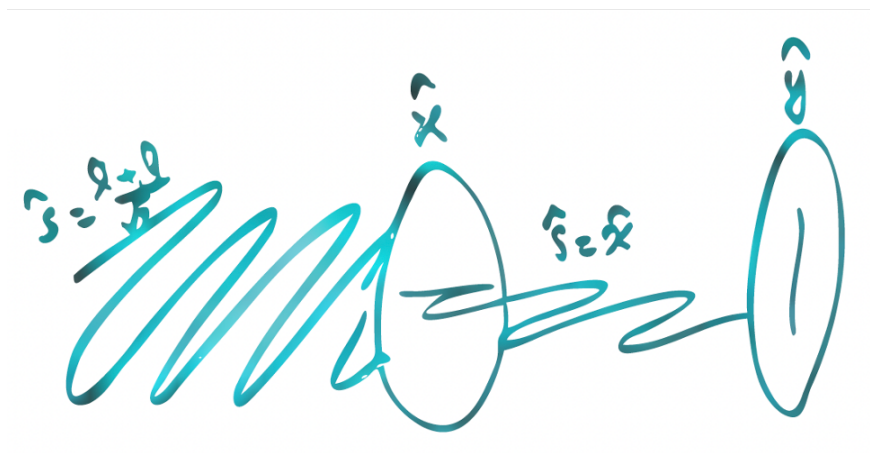
Figure 2: Light which first passes through an \hat{x} polarizer and then a \hat{y} polarizer.
