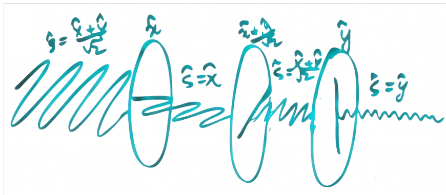
Figure 3: The same situation as in Figure 2, but with a \hat{n} = (\hat{x} + \hat{y})/\sqrt{2} polarizer inserted in between.
